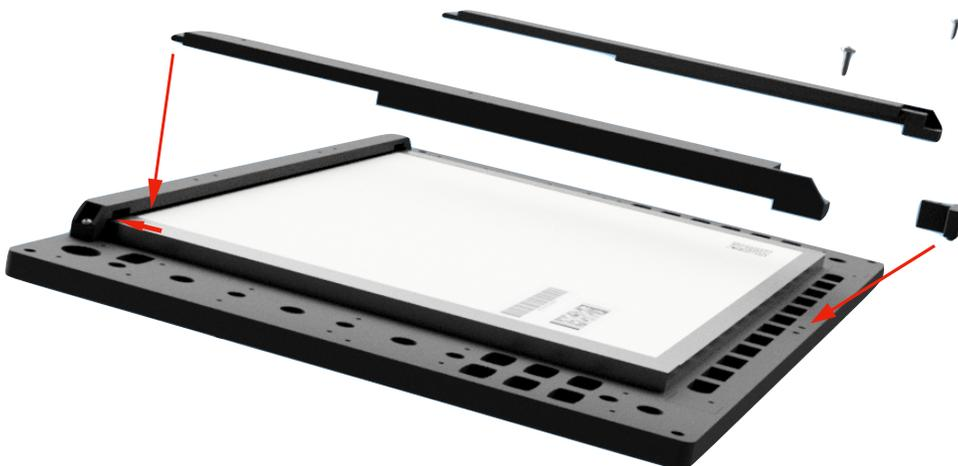
Glue the Bottom PCB holder onto the bottom face plate using locator pins for alignment
